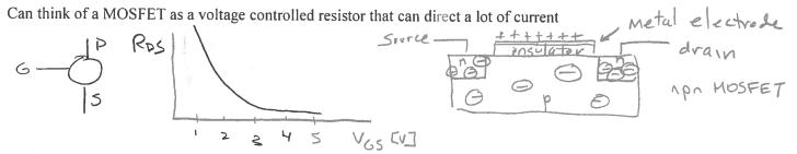
Notes: Input resistance is very high (therefore effectively no current goes into gate) Low-power MOSFETS are the "switches" used in computers (what is a switch?) MOSFETS are very sensitive to static electricity - use a grounding strap when you handle them in lab
